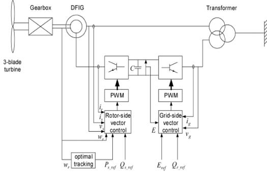
Fig.6 Vector control scheme for DFIG
