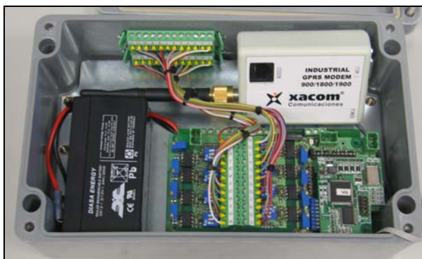
Fig. 8. Communication card for remote condition monitoring – communication via GPRS
