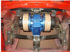
Fig. 9. Mechanical adaptation of the gearbox transmission to the chassis.
