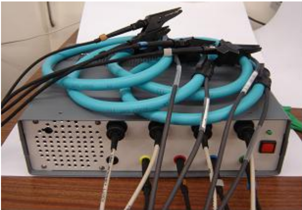
Fig. 2. Voltage terminals and current sensors connected to the Power Quality Monitor.
