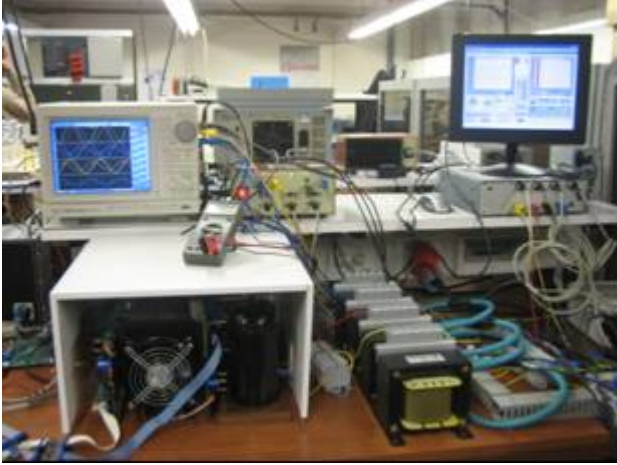
Fig. 4. Implemented laboratory prototype of the Shunt Active Power Filter with Power Quality Monitor.
