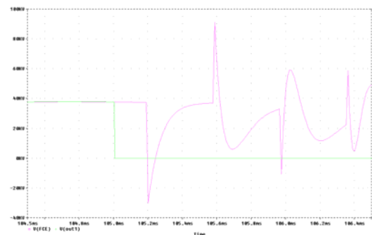
Fig. 5. Voltage waveform at supply substation (V (FCE)) after short-circuits at the end of the contact line.
