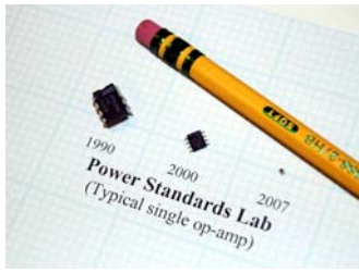
Figure 1: Reduction in component size. Smaller components reduce costs in several ways: smaller printed wiring boards, smaller plastic packages, even smaller power supply requirements. The packages shown are, from left, through-hole DIP, surface mount, and BGA or ball-grid-array.
