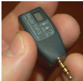
Figure 5. Probes for parameters that may be related to power quality are included: Temperature, Humidity, Barometric Pressure, etc. A GPS satellite receiver can ensure precise timing.
