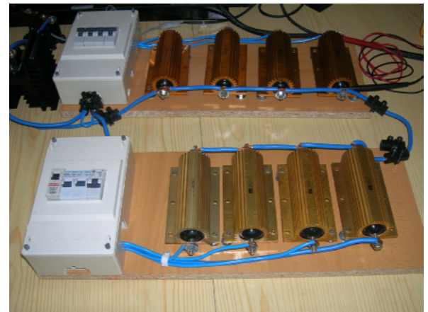
Figure 5. Resistances net to measure the internal equivalent resistance ( R_{int} ).
