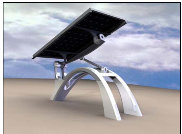
Fig. 6. Virtual prototype of the solar tracker.
