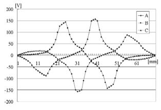
Fig. 3. Phase Voltage with the Sinusoidal Velocity
