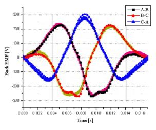
Fig. 11. Output voltage with no load
