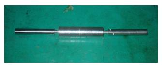
Fig. 9. Manufactured mover
