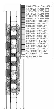
Fig. 2. Magnetic Flux Density of Tubular Linear Generator
