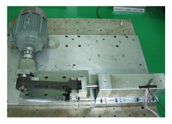
Fig. 10. Assembled linear generator and experimental setup.
