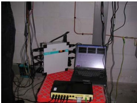
Fig. 5. Inasus Factory with the different instruments for make the comparison of the results of power quality measure.
