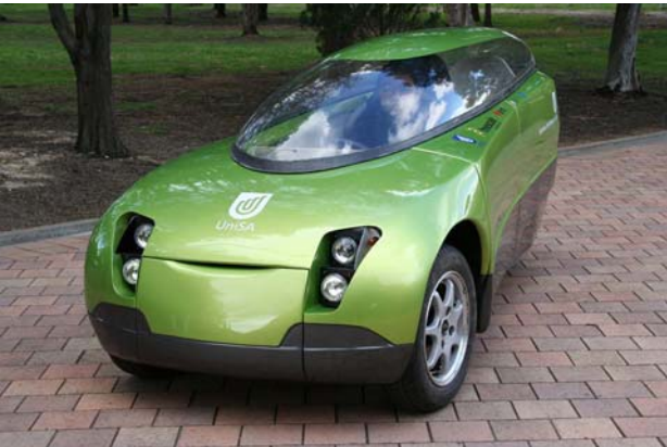
Fig. 7. Two-seater renewable energy vehicle: Trev, designed and built at the University of South Australia (Photo Credit: UniSA/World Solar Challenge)
