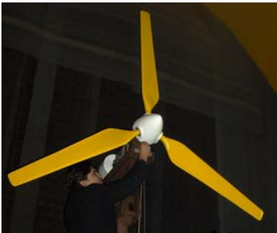
Fig.10-1kW wind turbine rotor on the testing platform
