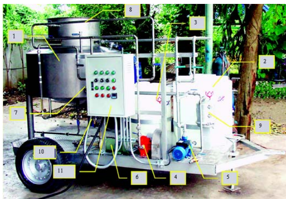
Figure 3 The biodiesel production unit.in Nhong Pling municipality, Nakorn Sawan province.
