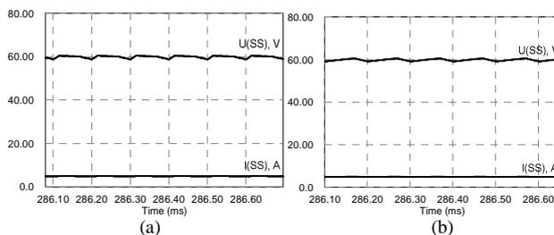
Fig. 10 Simulation results of the proposed converter during the SC discharging mode: SS side voltage ( $U_{SS}$ ) and current ( $I_{SS}$ ) at SC nominal (14.4 V) (a) and half of nominal (7.2 V) (b) voltage.
