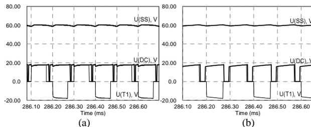
Fig. 9. Simulation results of the proposed converter during the SC discharging mode: DC-link voltage ( $U_{DC}$ ), transformer primary voltage ( $U_{TI}$ ), SS DC bus voltage ( $U_{SS}$ ), at SC nominal (14.4 V) (a) and half of nominal (7.2 V) (b) voltage.
