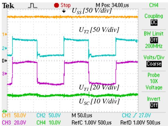
Fig. 13. General operating waveforms of the proposed bi-directional converter during the SC charging mode (SS side DC bus voltage  $U_{SS}$ , transformer secondary voltage  $U_{T2}$ , transformer winding voltage  $U_{T1}$ , SC voltage  $U_{SC}$ ).
