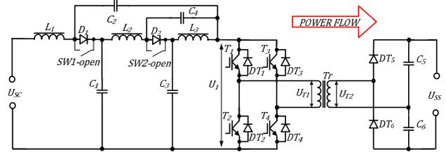
Fig. 3. Power circuit configuration in the discharging mode.
