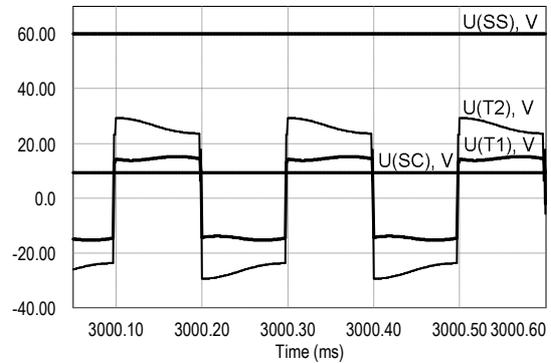
Fig. 5. Simulation results of the proposed converter during the SC charging mode: SS side DC bus voltage ( $U_{SS}$ ), transformer primary voltage ( $U_{T1}$ ), transformer secondary voltage ( $U_{T2}$ ), SC voltage ( $U_{SC}$ ).
