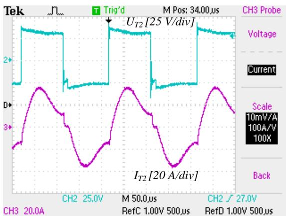
Fig. 14. Transformer secondary voltage ( $U_{T2}$ ) and current ( $I_{T2}$ ) waveforms.
