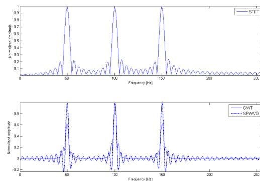
Fig. 14. Freq. profile comparison for STFT, GWT and SPWVD – linear amplitude scale (input parameters Table I point 3).
