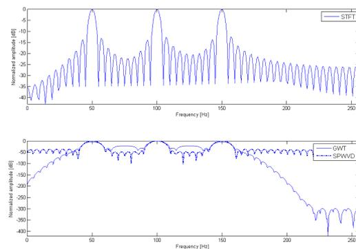
Fig. 13. Freq. profile comparison for STFT, GWT and SPWVD – decibel amplitude scale (input parameters Table I point 2).
