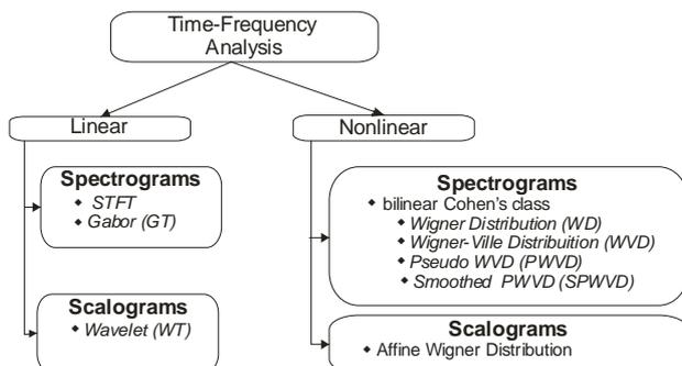
Fig. 3. One of the signal analysis classifications.
