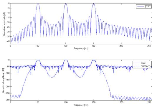
Fig. 17. Freq. profile comparison for STFT, GWT and SPWVD – decibel amplitude scale (input parameters Table I point 4).
