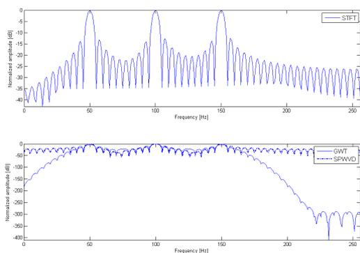
Fig. 11. Freq. profile comparison for STFT, GWT and SPWVD – decibel amplitude scale (input parameters Table I point 1).
