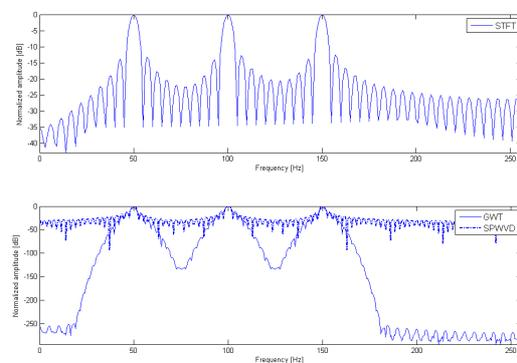
Fig. 15. Freq. profile comparison for STFT, GWT and SPWVD – decibel amplitude scale (input parameters Table I point 3).
