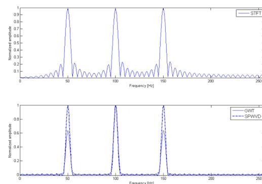
Fig. 16. Freq. profile comparison for STFT, GWT and SPWVD – linear amplitude scale (input parameters Table I point 4).
