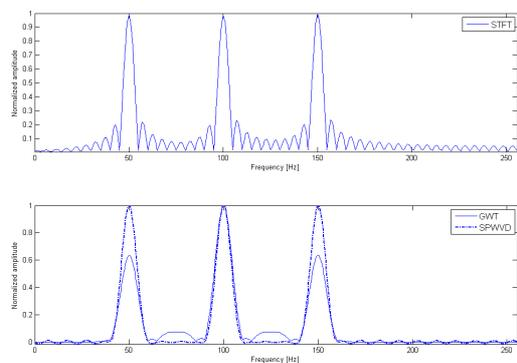
Fig. 12. Freq. profile comparison for STFT, GWT and SPWVD – linear amplitude scale (input parameters Table I point 2).
