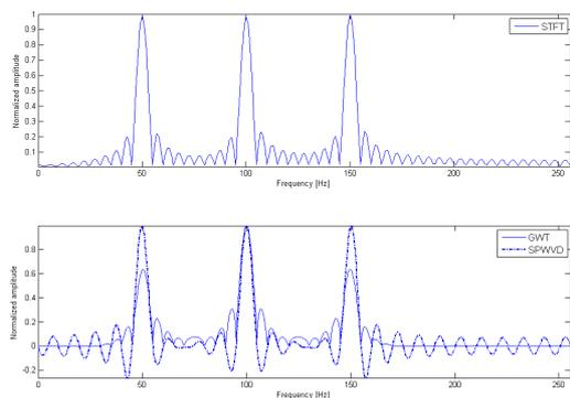
Fig. 10. Freq. profile comparison for STFT, GWT and SPWVD – linear amplitude scale (input parameters Table I point 1).
