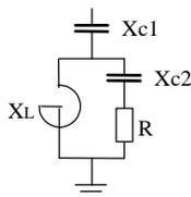
Fig. 1. Schematic diagram of the third-order filter.
