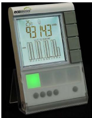
Fig.10. Inhome Display Unit - ecoMeter
