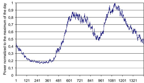
a) Measured load curve
