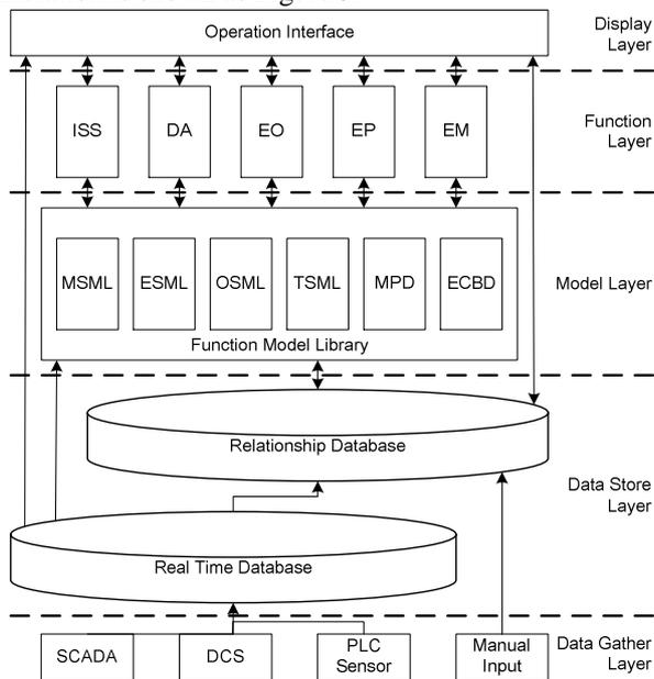
Fig.5. Online simulation software architecture
