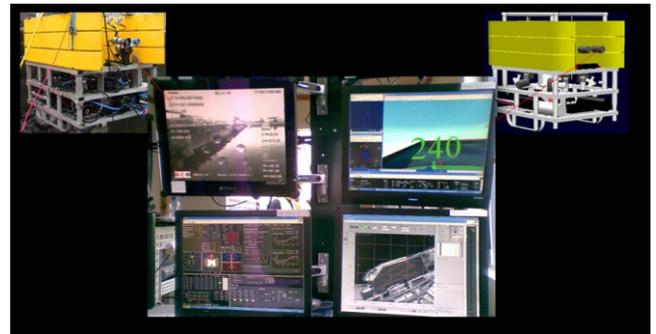
Fig. 12. Control Cabin: comparison of views from real and virtual pilot cameras
