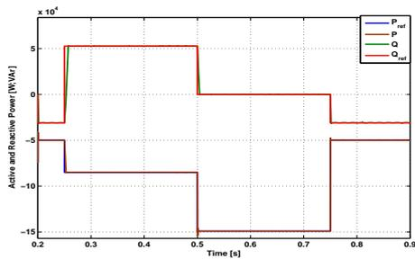
Figure 8. Response of step tests for active and reactive power with parameters variations in several speed operation.
