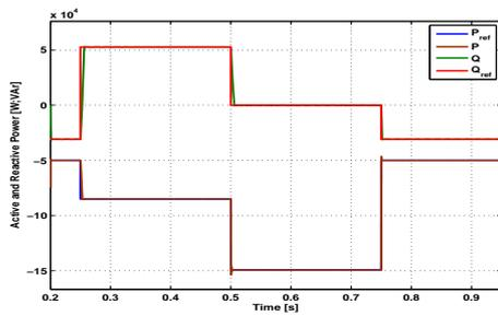
Figure 6. Response of step tests for active and reactive power in several speed operation.
