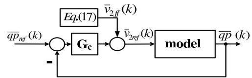
Figure 2. Decoupling and deadbeat control block diagram.
