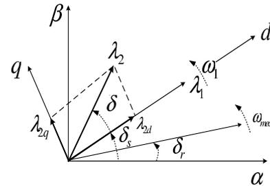
Figure 1. Stator and rotor flux vectors in the synchronous dq frames.
