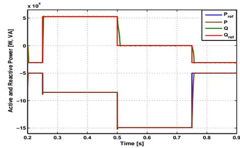
Figure 4. Response of step tests for active and reactive power and rotor currents in supersynchronous operation.
