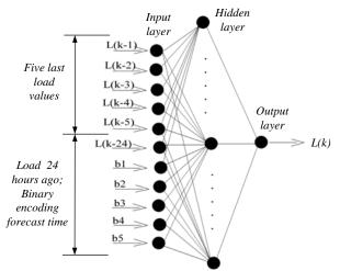
Fig. 2. Simplified ANN architecture used to forecast hourly load.
