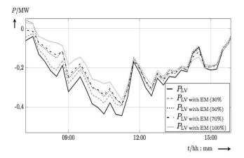
Fig. 5 daily progression of the power at the low voltage transformer ( $P_{LV}$ ) without and with energy management including different percentages of integrated storages systems in the grid ( $P_{LV \text{ with EM (30 \%)}}$ ,  $P_{LV \text{ with EM (50 \%)}}$ ,  $P_{LV \text{ with EM (70 \%)}}$ ,  $P_{LV \text{ with EM (70 \%)}}$ )
