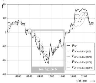
Fig. 4. daily progression of the power at the low voltage transformer ( $P_{LV}$ ) without and with energy management including different percentages of integrated storages systems in the grid ( $P_{LV}$  with EM (30 %),  $P_{LV}$  with EM (50 %),  $P_{LV}$  with EM (70 %),  $P_{LV}$  with EM (100 %))
