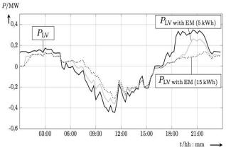
Fig. 3. daily progression of the power at the low voltage transformer ( $P_{LV}$ ) without energy management and with energy management including different storage capacitys ( $P_{LV \text{ with EM}}$  (5 kWh),  $P_{LV \text{ with EM}}$  (15 kWh))
