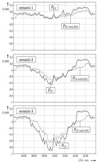
Fig. 1. daily progression of the power of the low voltage grid transformer without energy management  $(P_{\rm LV})$  and with it  $(P_{\rm LV})$  with EM) in three different scenarios of photocoltiac system integration
