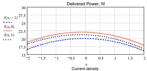
Fig. 5 Fuel Cell delivered power versus current density for three levels of mechanical compression
