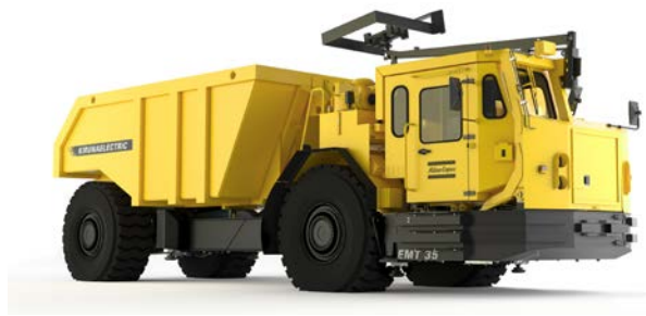
Fig. 2. Trolley powered EMT-35 truck (Courtesy of Atlas Copco)
