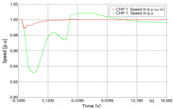
Fig 11. Frequency after disconnection with and without 3 RTs.
