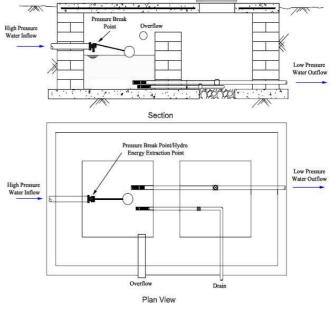
Fig.2 Typical Break Pressure Tank
