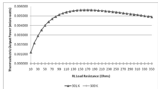
Fig. 9. The electrical power generated at the load resistor (RL) with a temperature gradient of 1 Kelvin between both sides of the device
