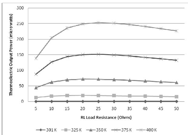
Fig. 11. The electrical power generated at the load resistor (RL) with different temperature settings applied to the thermal contact connected to Copper 1, and a doping level of  $1e^{+16}cm^{-3}$  for both P-type and N-type pellets
