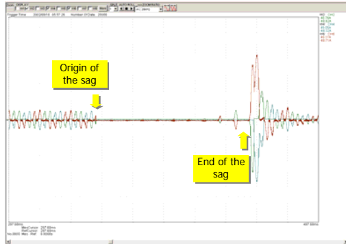
Fig. 26. Waveforms of the supply line currents during the sag
