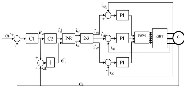
Figure 1. Classic scalar control of an induction machine.
