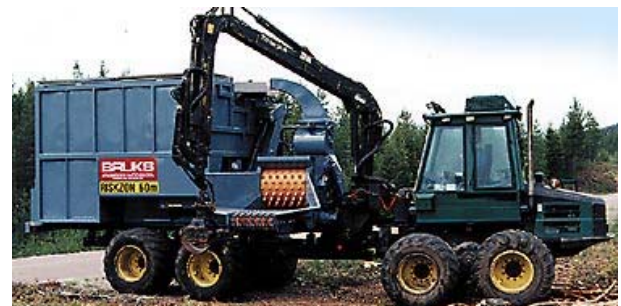
Fig 6.- Movable chipped machine
