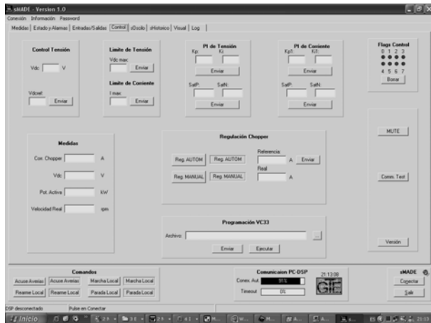
Fig. 17. PC monitor program interface (control section)
