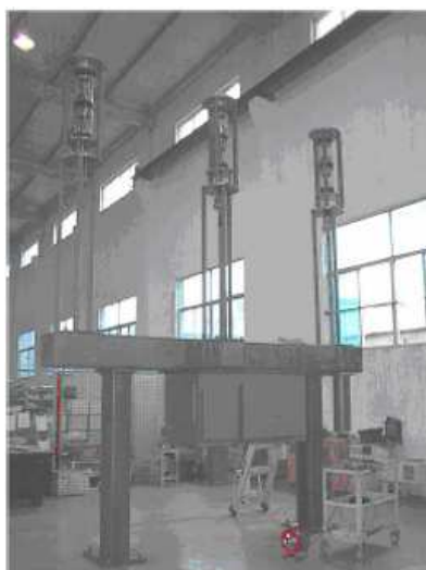
Figure 13. Single-break 126kV/40kA/2kA VCB [11]
