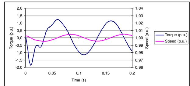
Fig. 7. Torque and speed oscillations of the synchronous machine SM<sub>1</sub>.
