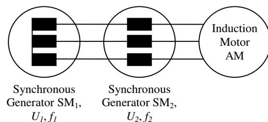
Fig. 2. Schematics of the two-frequency method comprising two synchronous generators.
