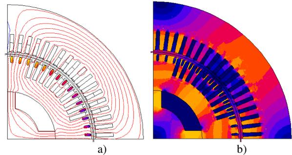
Fig. 6. Synchronous machine SM<sub>1</sub>, current density in the damper (a) and magnetic flux density (b).
