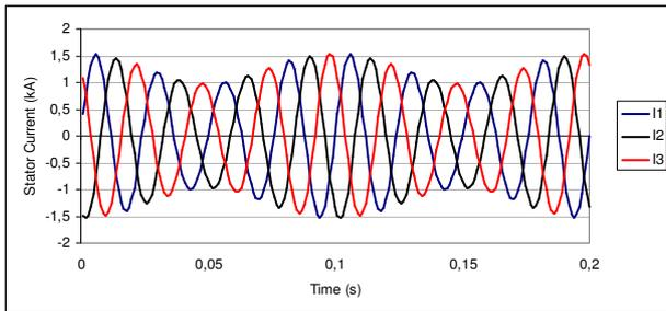
Fig. 4. Stator currents of AM and both SMs.
