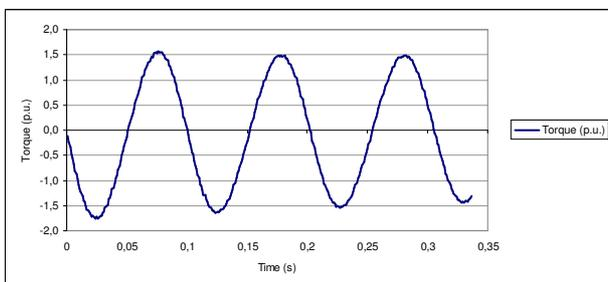
Fig. 5. Torque oscillations of the asynchronous machine.
