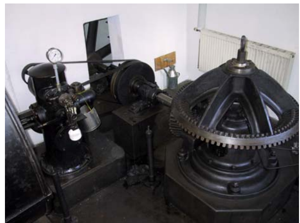
Fig. 2. Bevel gear pair used as speed increaser in a small hydro power station
