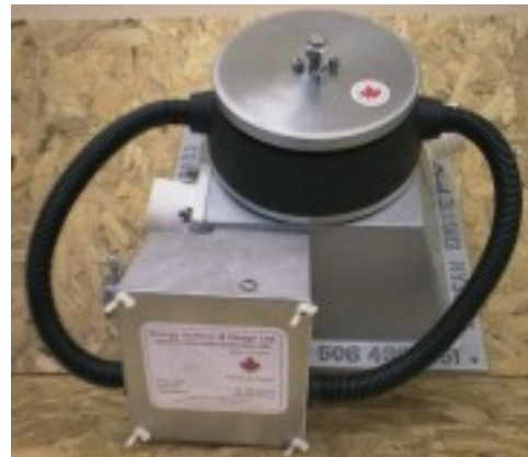
Fig. 1. Turgo water turbine connected directly to the generator
