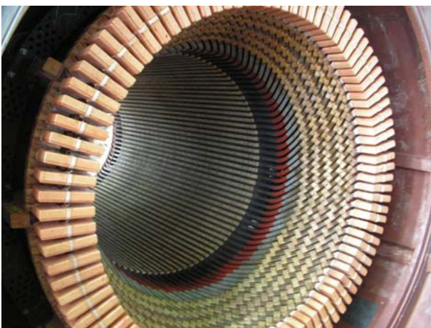
Fig.6. Stator with winding of the asynchronized compensator 100 Mvar
