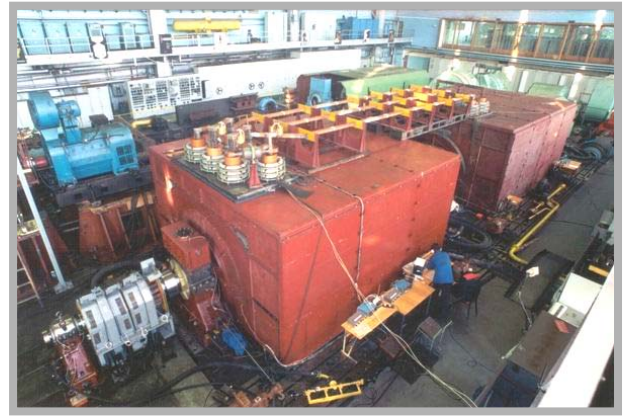
Fig. 7. Type T3Φ-110-2 asynchronous turbogenerator at the rig tests under the back-to-back loading duty.
