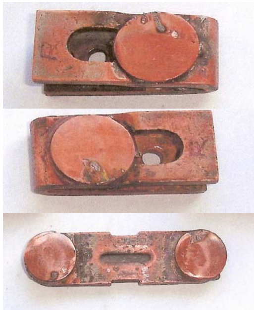
Figure 5 - The aspect of fix and mobile contacts after tests
